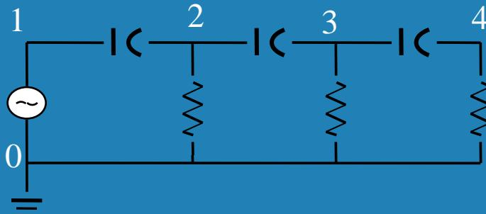
\*AC8.CIR - Multi-stage high pass circuit
